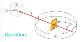
In 1909, Rutherford devised an experiment using an extremely thin sheet of gold foil coated with zinc sulfide. He used gold foil because it could be hammered very thinly. He bombarded the foil with very small positive alpha particles from decaying radium, expecting them all to pass through the foil. Most did, but some were deflected at angles to the foil.
