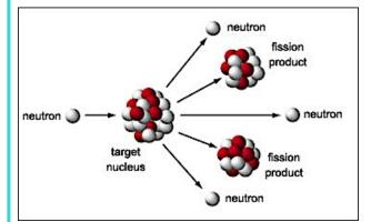
Nuclear fission is the splitting of atomic nuclei. There are two fissionable substances in common use in nuclear reactors: uranium 235 and plutonium 239. For fission to occur, the uranium 235/plutonium 239 nucleus must first absorb a neutron. The nucleus undergoing fission splits into 2 smaller nuclei and 2/3 neutrons and energy are released. The neutrons may go on to start a chain reaction.
