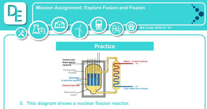
a) What is the role of the control rods in the reactor?
